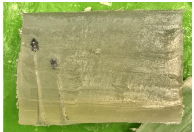
Fig. 3: Comparison of penetration depths of two pellet types Source: created by the authors
