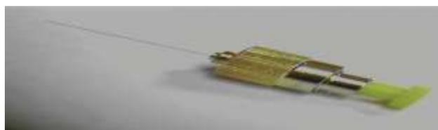
Fig. 4 (on-line color) Photo of packed sensor (mainly, connected piece of the fiber with 25 mm length to FBG along the fiber length out of connection), [7].
