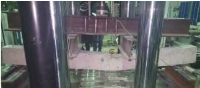
Figure 14. Beam in its ultimate configuration.
