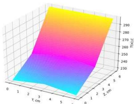
Figure 13. The law of distribution of non-temperature on the face (1, 3, 5, 7) of the cube at  $m = 2$  for the non-insulated case.
