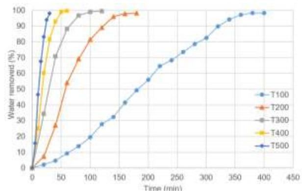
Figure 3. The behavior of the Water removed as a function of the time
