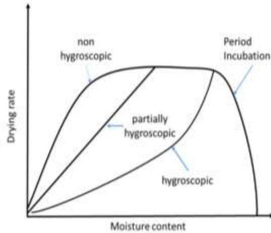
Figure 6. Different stages of the lateritic mineral drying process.
