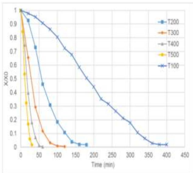
Figure 4. The behavior of the Water removed as a function of the time.
