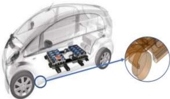
Figure 1. Battery module placement and the door sill area, [11]
