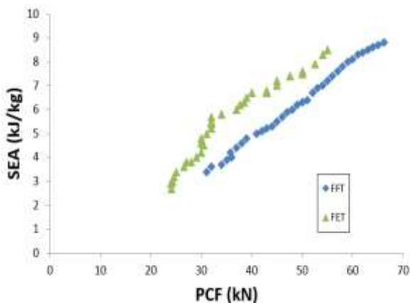
Figure 10. Pareto fronts for the double cylindrical tubes
