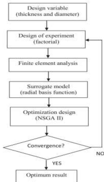
Figure 4. The multi-objective optimization design flowchart
