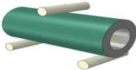
Figure 3. The FE model geometry for a double tube filled with foam
