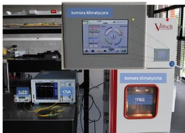
Figure 12. Laboratory stand for measuring TFBG temperature
