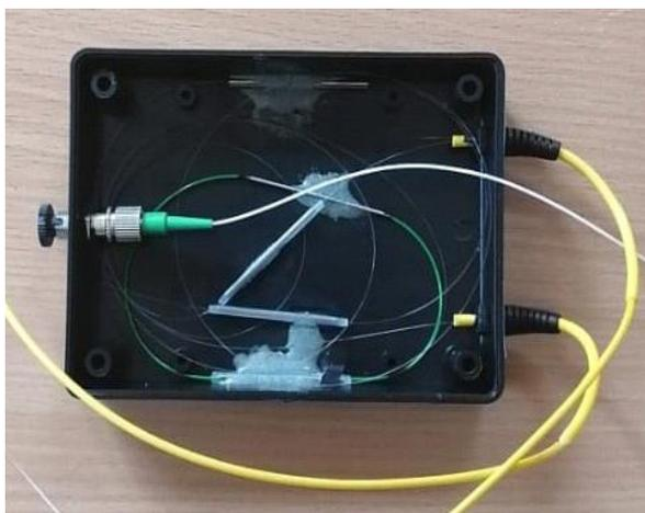
Figure 10. Conventional Bragg fiber-optic sensor
