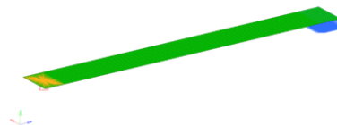
Fig. 7 FEM for the analysis of damping properties
