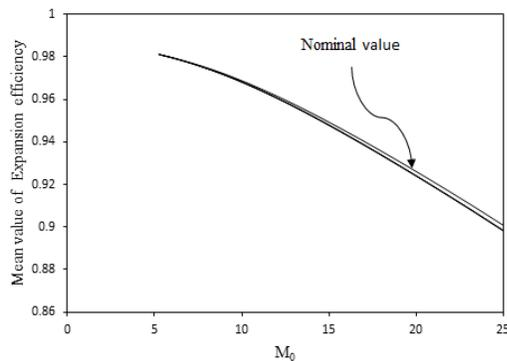
Fig 10 Mean Expansion Efficiency for N different points of each of the uncertain parameters Changes with Fly Mach
