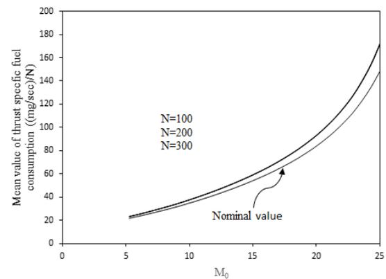
Fig 6 Mean specific fuel consumption for N different points of each of the uncertain parameters Changes with Fly Mach
