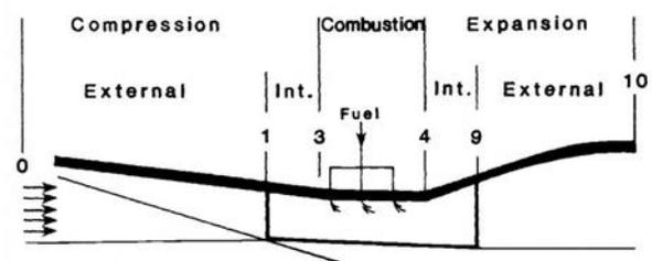
Fig 2 Sections of the Scramjet air breathing Engine
