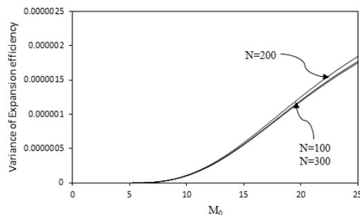
Fig 11 Variance of expansion efficiency for N different points of each of the uncertain parameters Changes with Fly Mach
