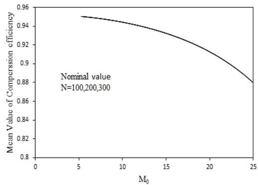
Fig 12 Mean compression efficiency for N different points of each of the uncertain parameters Changes with Fly Mach
