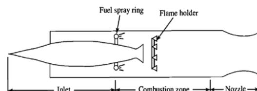
Fig 1 schematic diagram of a ramjet
