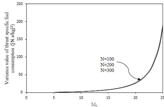
Fig 7 Variance of specific fuel consumption for N different points of each of the uncertain parameters Changes with Fly Mach
