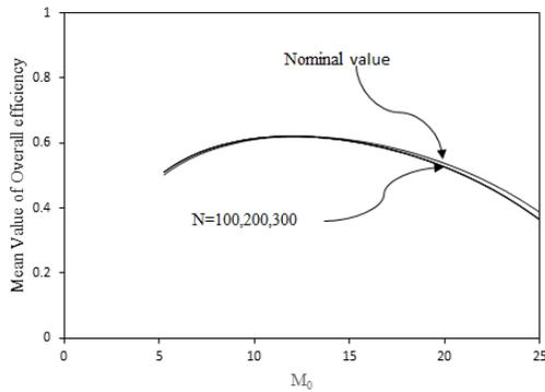
Fig 8 Mean overall efficiency for N different points of each of the uncertain parameters Changes with Fly Mach
