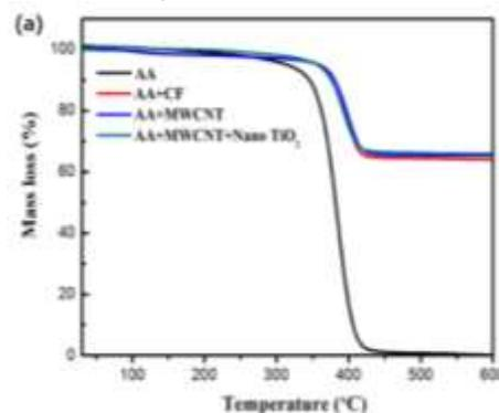
(a) Thermal mass loss curve
