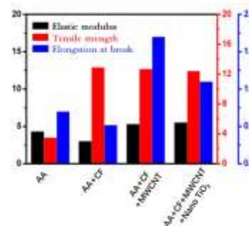
( b ) Elastic modulus, tensile strength, and elongation at break of anti-corona coating film
