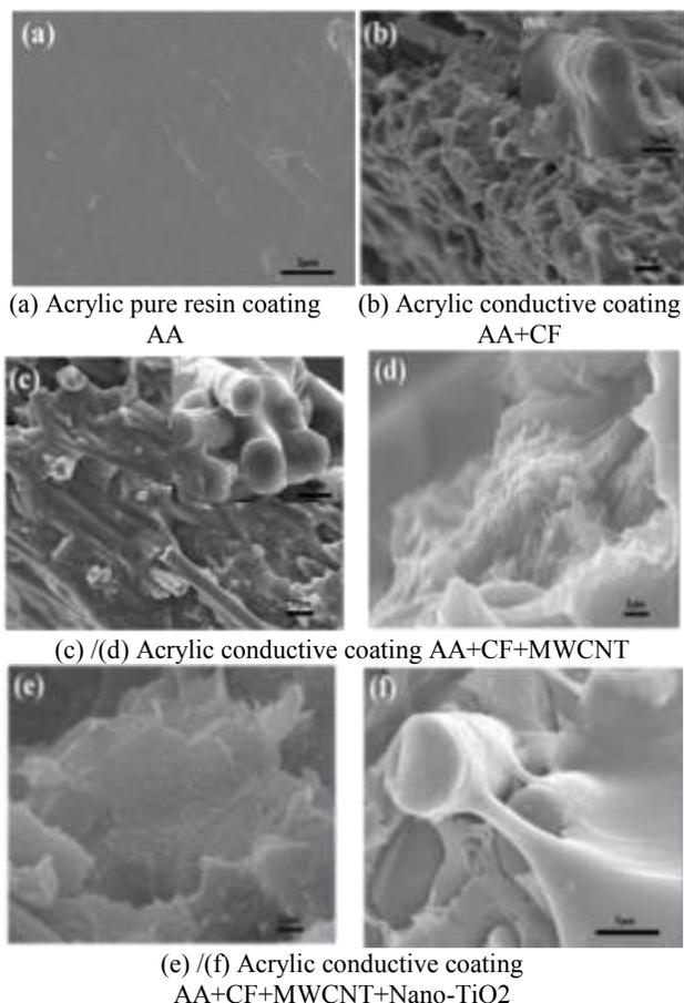
Fig. 4 SEM images of brittle sections of four anti-corona coatings
