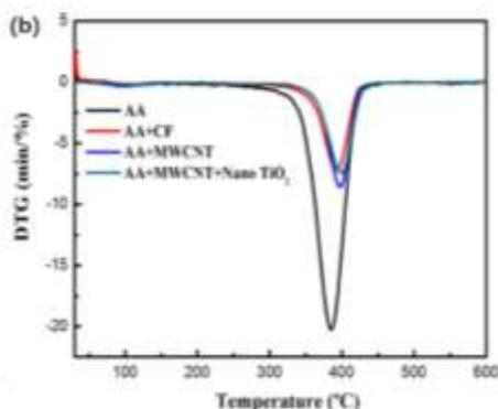
(b) Derivative thermogravimetric (DTG) curve
