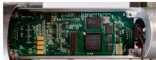
(c) the monitoring node's FPGA board
